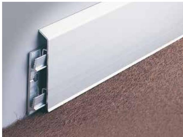
This anodized aluminium skirting profile is easy to install and can also be used to conceal cables or protect wires while providing an elegant baseboard finish. The internal interlocking support piece is fixed to the wall with screws. This profile is ideal for office environments that have both aesthetic requirements and require solutions for telephone and computer wire passage.
